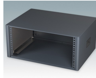
M6619544 TECHNOMET 19" 5Ux400mm Aluminium Anthracite RAL 7016 244.5x539x400mm
